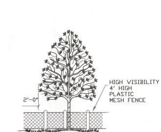
TREE PROTECTION SCALE: N.T.S. DURING CONSTRUCTION
