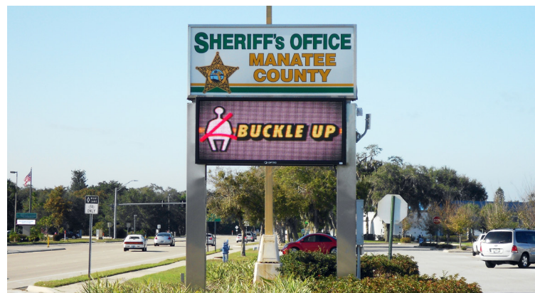
IMPACT-RGB: 12mm pixel pitch (3'-5" x 8')
