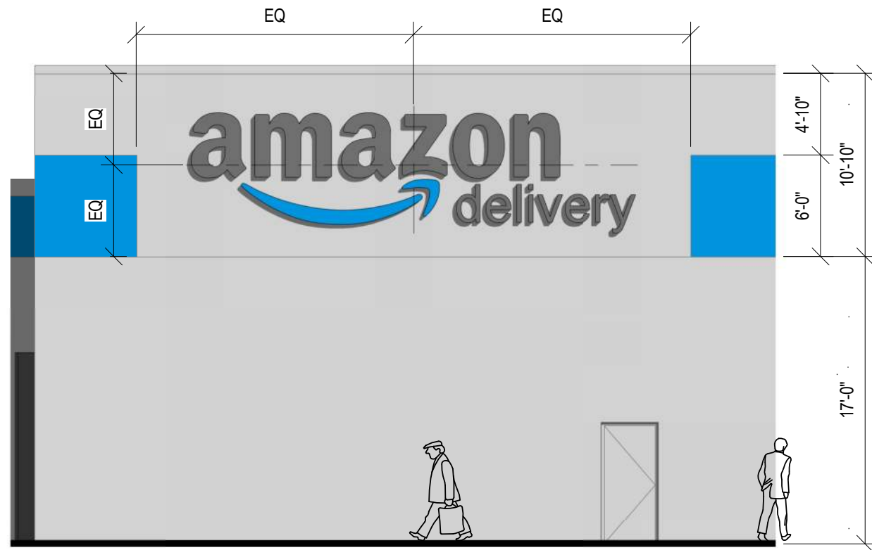
MAIN BUILDING SIGN ELEVATION
