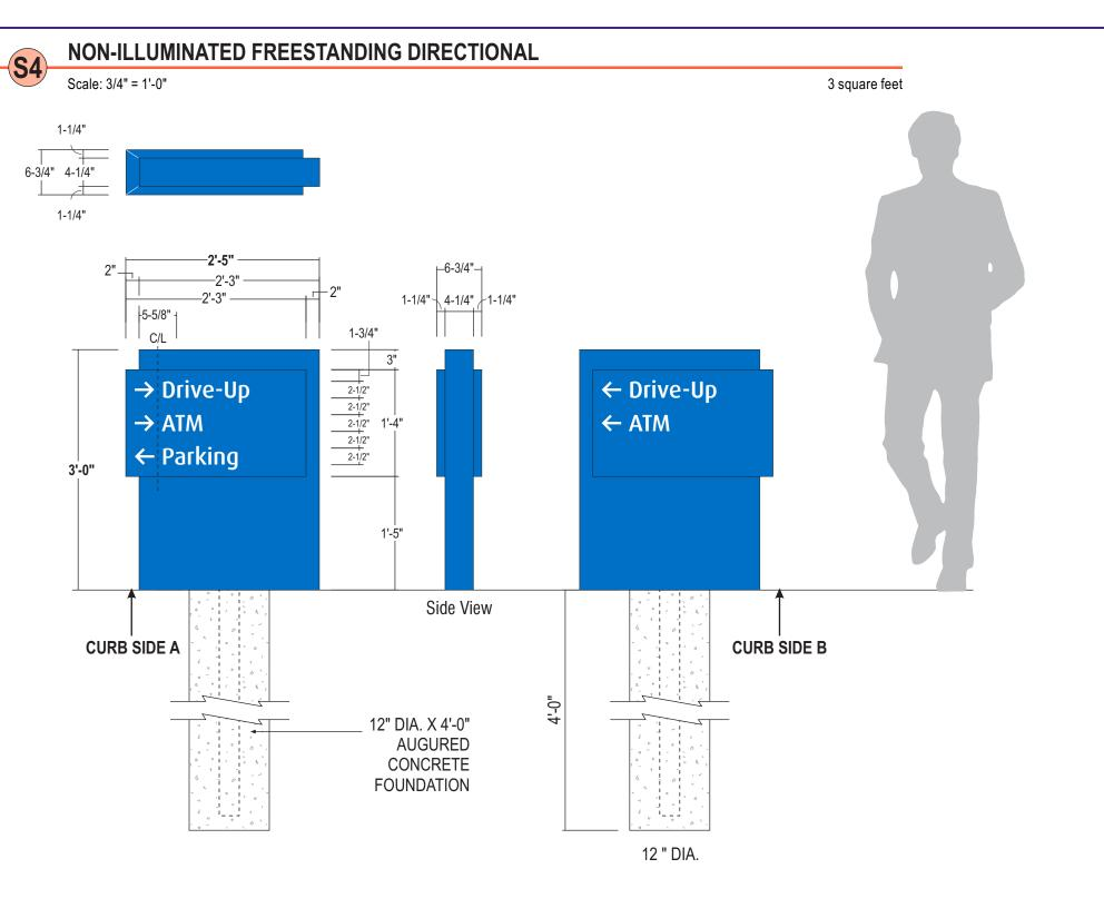
**SURROUND:** Fabricated alum. 4-1/4" total depth w/ 4" x 1-1/2" x 1/8" alum. channel; skinned with .090 alum. painted White semi gloss finish
