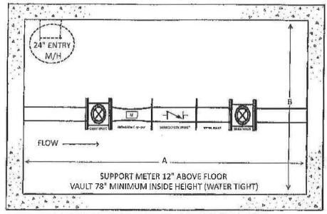
\* SWING CHECK VALVE IS ONLY NETDED WITH INTERCONNECTES MULTIPLE MEITER FITS TO PREVENT REVERSE FLOW SWING CHECKS SHOULD BE SMITH COUPER BRAND OR EQUIVALENT QUALITY AND FLOW CHARACTERISTICS. UPDATED 4:13-2022 MG
