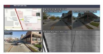
The RAS Video Logger allows the Village to load pavement and ROW imagery for a specific location within the Village and sequentially travel down the roadway. In addition, the Video Logger houses the Ladybug Panoramic ROW imagery (all 5 views), LCMS downward pavement imagery, PCI scores, and right of way inventories.
