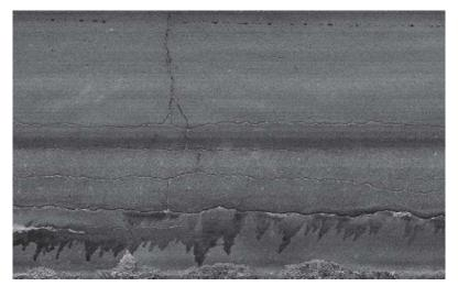
100% linear assessment of the roads, in accordance with guidelines within the **ASTM D6433**, **ASTM E1656**, and **ASTM E3303**. This methodology removes the subjectivity of rating small sample areas of the road segment where the sample may not represent the condition of the entire roadway segment.
