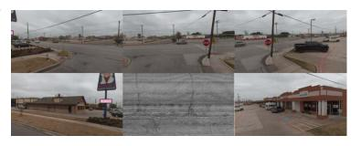
right-of-way (ROW) assets for extraction. The images will be collected as a 360-degree right-of-way panorama, including forward, rearward, and downward pavement viewing images. Each image will be geolocated with at least 1 foot accuracy and delivered in ESRI file geodatabase format.
