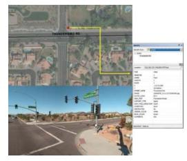
asset that can be identified in the images. Other common roadside features for capture include sidewalks, pavement markings/striping, pedestrian curb ramps, curb/gutter, traffic signals, streetlights, fire hydrants, bus stop shelters, medians, and many others.
