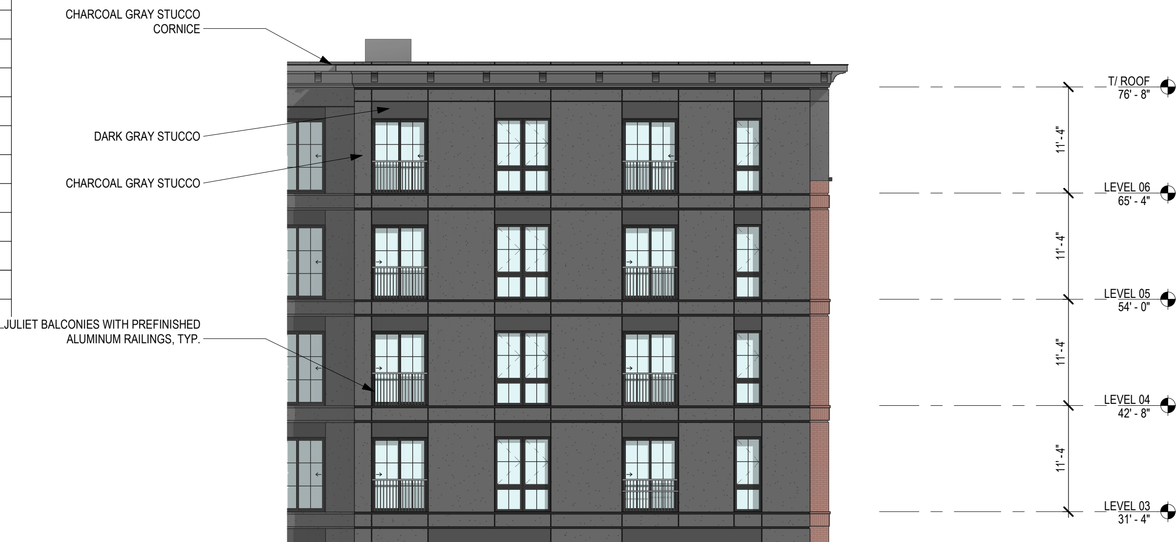
3 SOUTH COURTYARD EAST ELEVATION SCALE: 1" = 10'-0"
