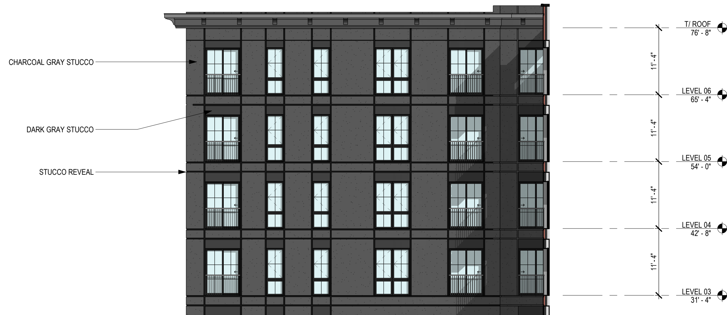
4 SOUTH COURTYARD WEST ELEVATION SCALE: 1" = 10'-0"
