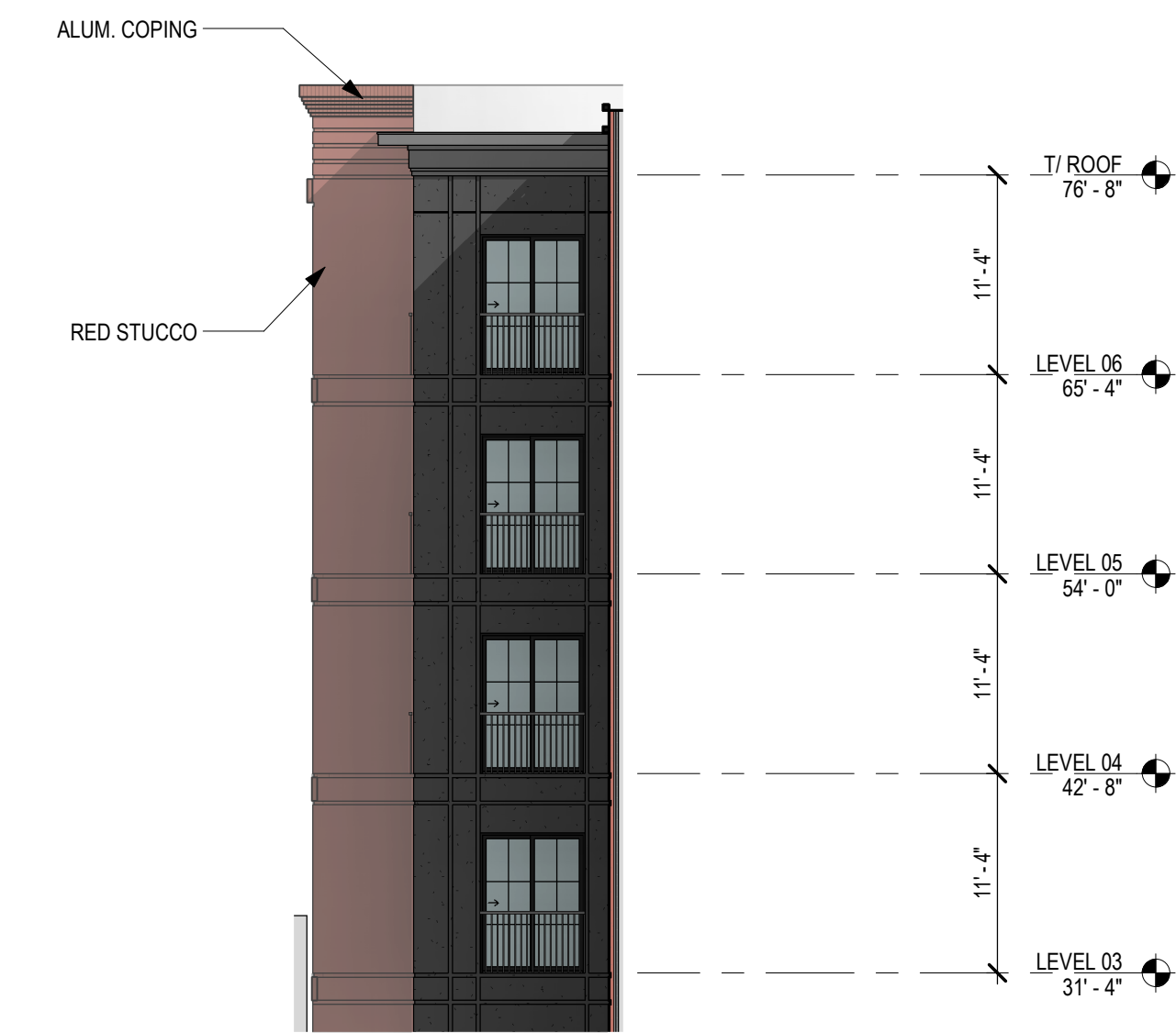
1 NORTH COURTYARD EAST ELEVATION SCALE: 1" = 10'-0"
