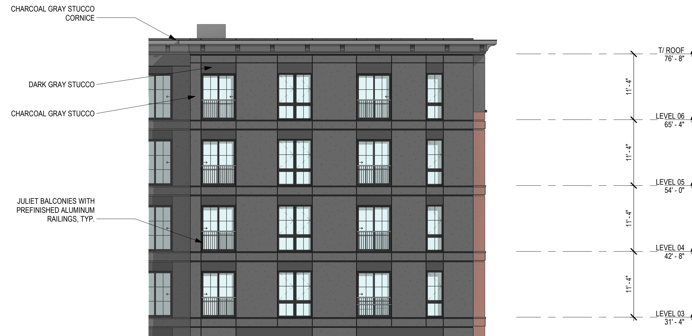
3 SOUTH COURTYARD EAST ELEVATION SCALE: 1" = 10'-0"
