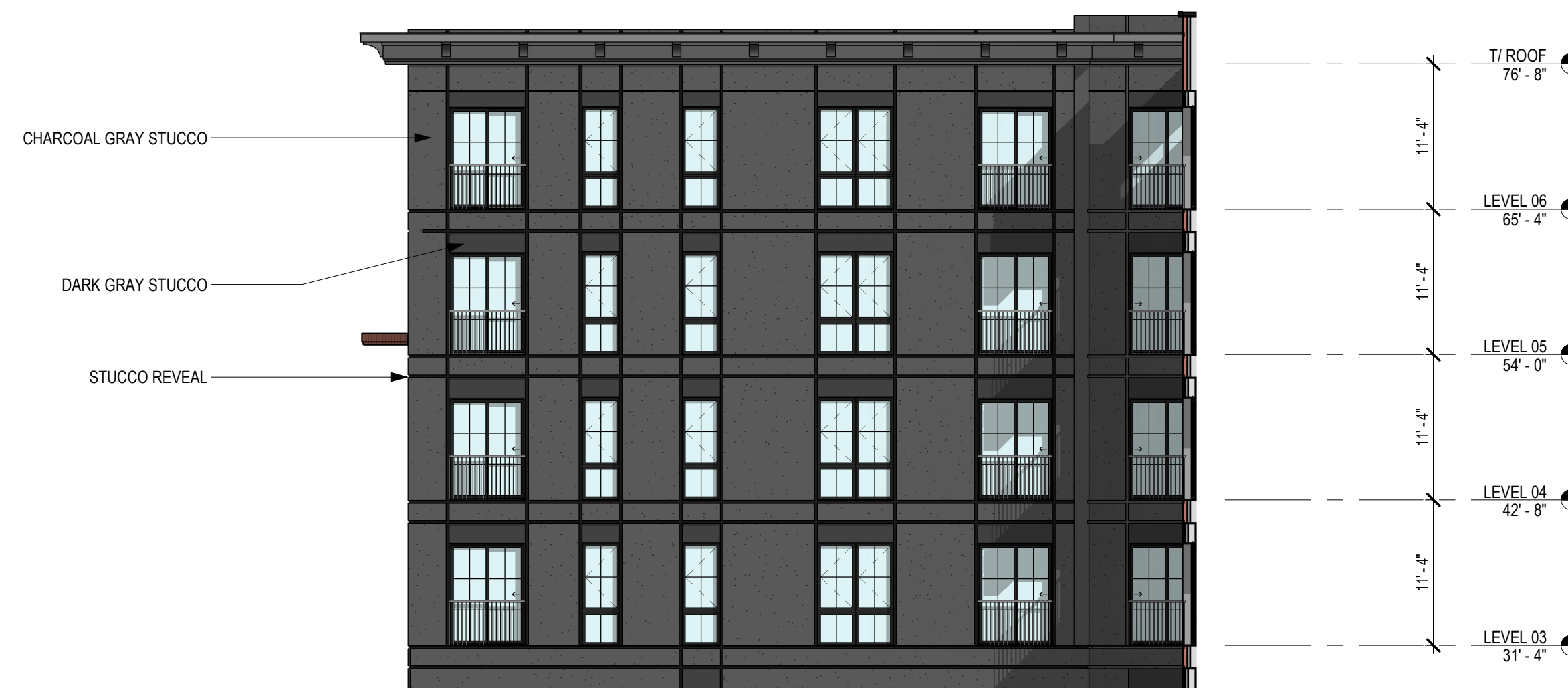
4 SOUTH COURTYARD WEST ELEVATION SCALE: 1" = 10'-0"
