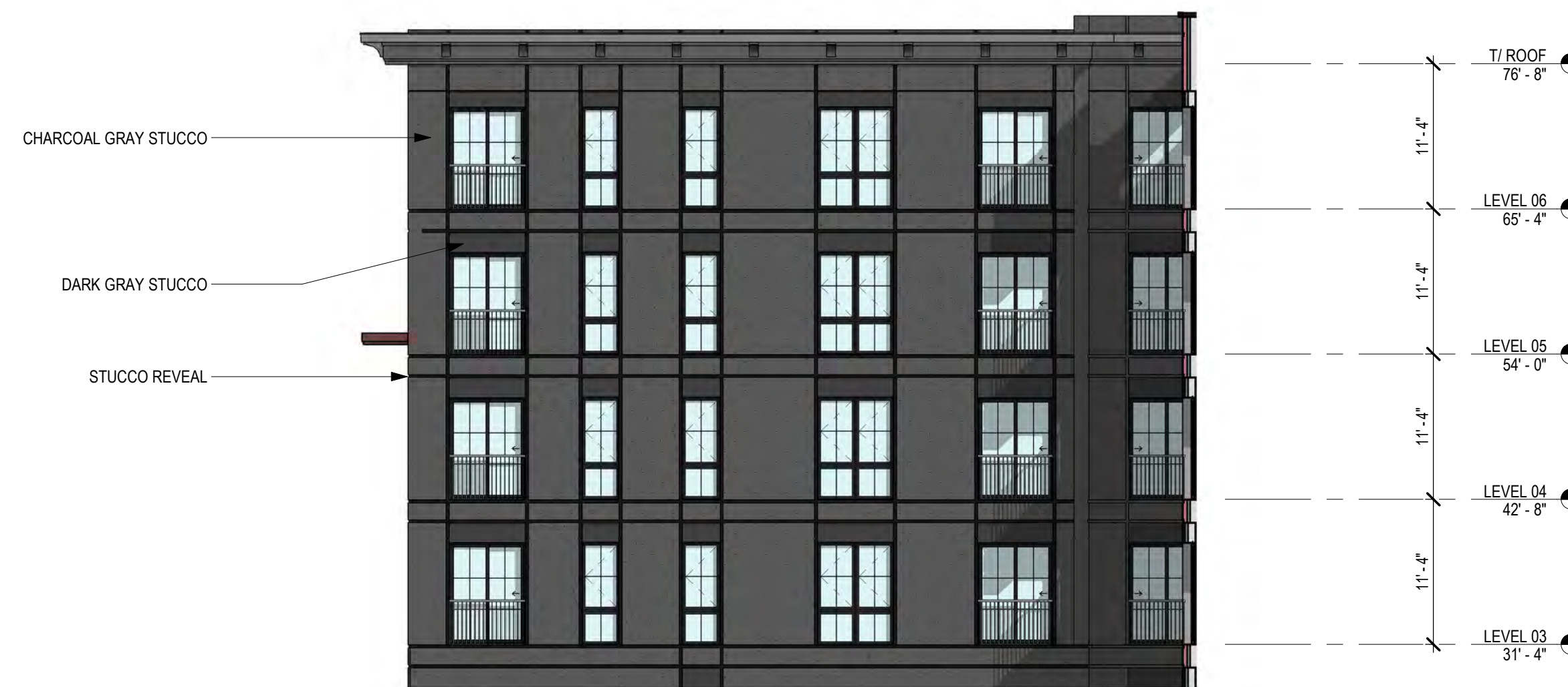
4 SOUTH COURTYARD WEST ELEVATION SCALE: 1" = 10'-0"
