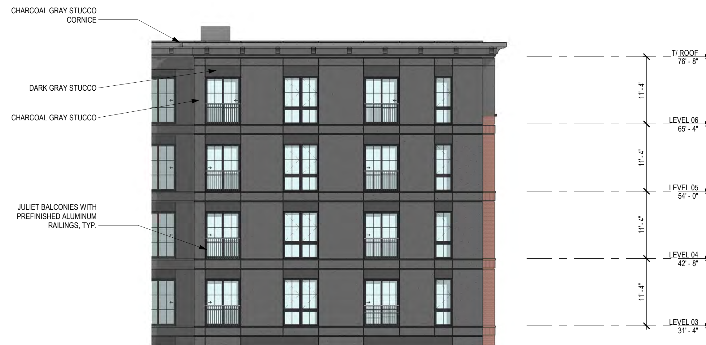
3 SOUTH COURTYARD EAST ELEVATION SCALE: 1" = 10'-0"
