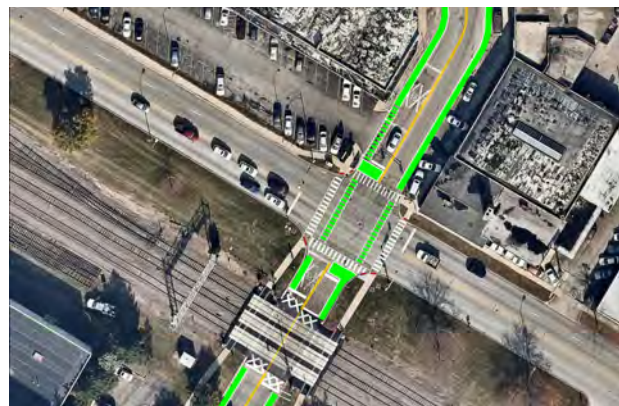
Figure 4.87 - Walnut/Ridge at Northwest Highway, Intersection / Bikeway Design Concept
